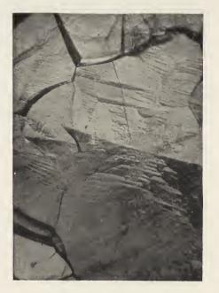
Fig. 5. (x 35 Diameters. Vertical Illumination.) Dendrites on Surface of Silver.
